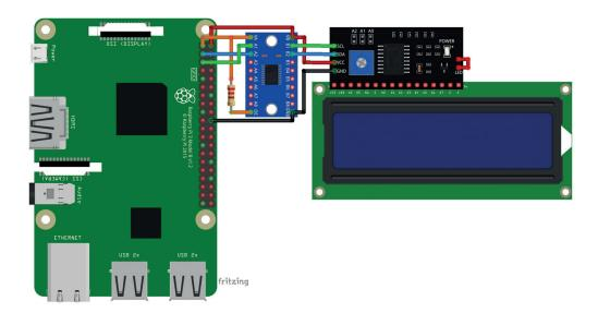
Please note that to use HD44780 20x04 LCD Display I2C bundle with Raspberry Pi, using Logic Level Converter is needed, which you can also pick up from our catalog.
