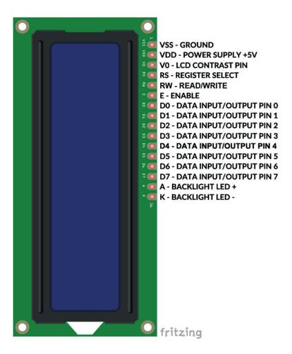
The VO pin uses analog voltage to set up the screen contrast level. Hardware contrast adjustment can be done by using voltage divider or potentiometer.
